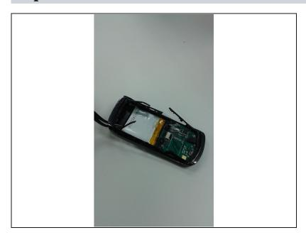
Use the tweezers to pry off the black and silver plastic that lines the edges of the device.
