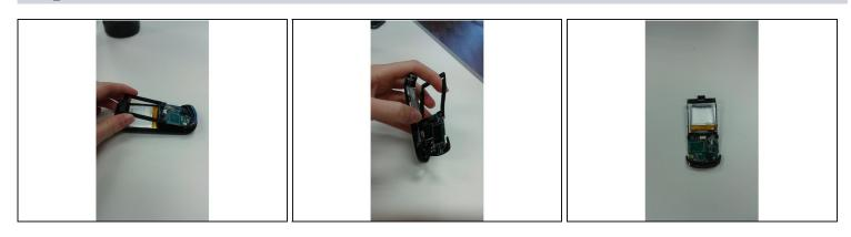
• Lift up to remove the black plastic outline that fits within the back cover. This will be connected to the main board and battery.
