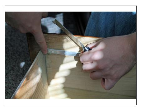
Wait until the putty has almost completely dried (approximately 30 minutes), at which point use the reference points and replace the brace bar, sliding in from the top of the drawer.
