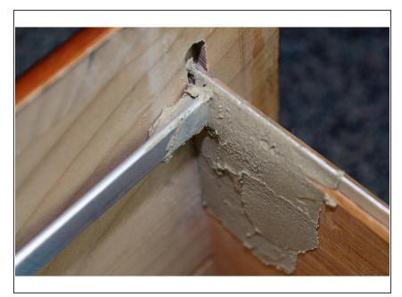
Reinforce the brace bar once you have properly placed it in the drawer front with wood putty to ensure stability.
