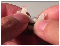
• Remove the plastic casing from the underside of the blade.
