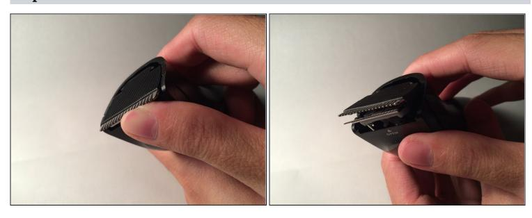
Place thumb underneath the blade; push upward to pop the blade off.
