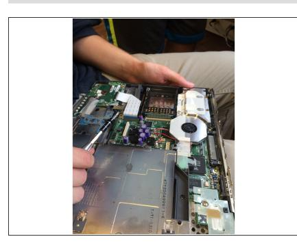
The entire green plank that spans the bottom of the laptop, including underneath the other pieces shown above is the motherboard.
