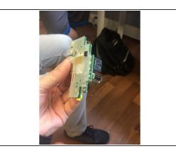
Unscrew and remove the power/USB card using the Phillips head #00 screwdriver. The power/USB card is the white plastic piece in the bottom corner of the laptop, shown in the picture.
