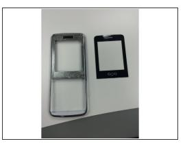
Use the needle nose pliers to pull the screen away from the front of the disassembled phone.
