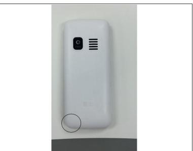
Insert your thumb into the groove on the back lefthand corner of the phone to unsnap the back cover.
