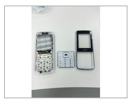
Once the front and back of the phone are separated, push the keypad out of the front portion of the phone.
