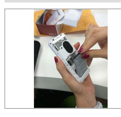
Remove the battery from the back of the phone.
