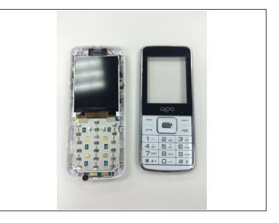
• Use the plastic opening tool to pry the front of the phone away from the back of the phone.
