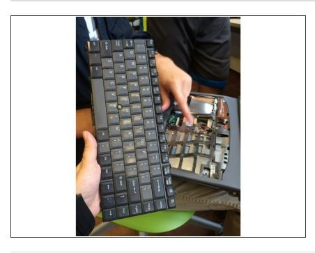
Once the keyboard is unplugged, gently pull it off. It should easily remove from the laptop. Replace this with the new keyboard. Plug the new keyboard in and replace the plastic panel.
