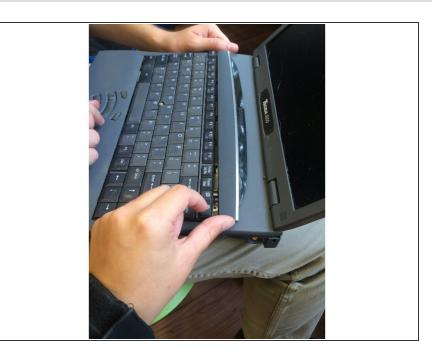
Locate the long, thin plastic panel above the keyboard. This panel is positioned between the top of the keyboard and the screen of the laptop.
