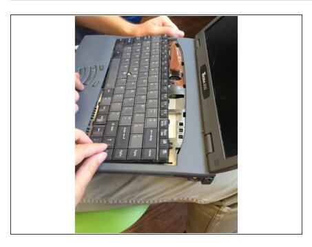
Removing the panel will reveal a plug that connects the keyboard to the motherboard. Disconnect this plug.
