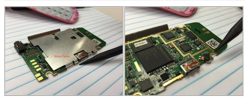
• Using tweezers and wedge, remove silver piece from green circuit board.
