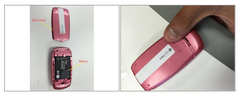
• Remove the back cover by pressing on the top middle raised lines of the back cover and sliding the cover off.
