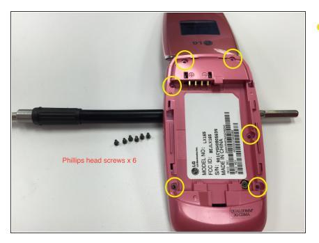
Use appropriately sized Philips-head screwdriver to remove the six small screws on the back of the phone under the battery.
