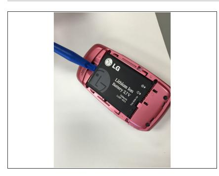
• Remove the battery by popping the top out and removing the battery.
