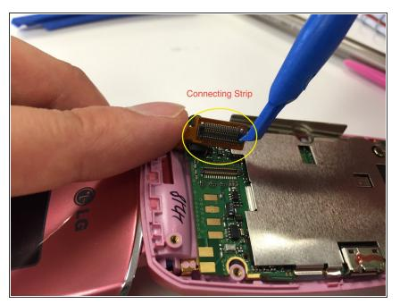
Use an opening tool to pop the orange connecting strip off of the circuit board.
