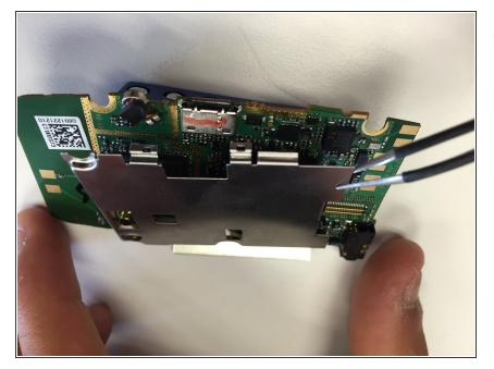
• Un-clip the 2 metal clips on one side of the circuit board.
