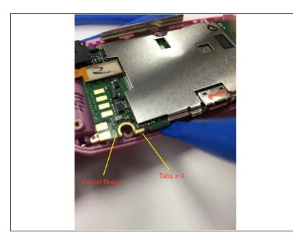
Use an opening tool to separate the tabs on the green circuit board from the front body of the phone.
