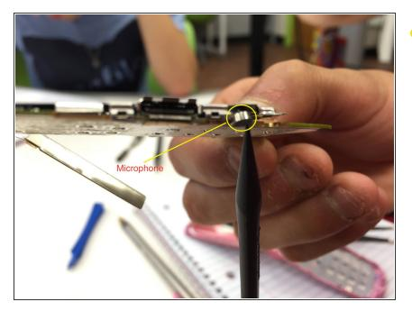
Remove the microphone (rip soldering).
