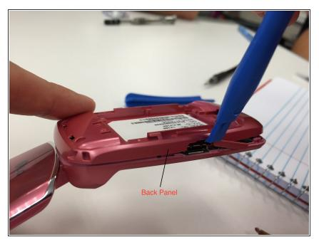
• Use an opening tool to pop the back panel apart around the edges, and then pry the whole piece off.
