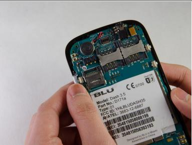
Remove volume and lock buttons by lifting them gently from the casing.
