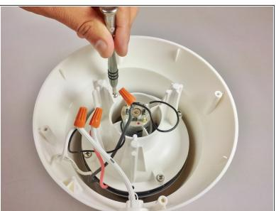
Remove the four 13 mm Phillips #2 screws.
