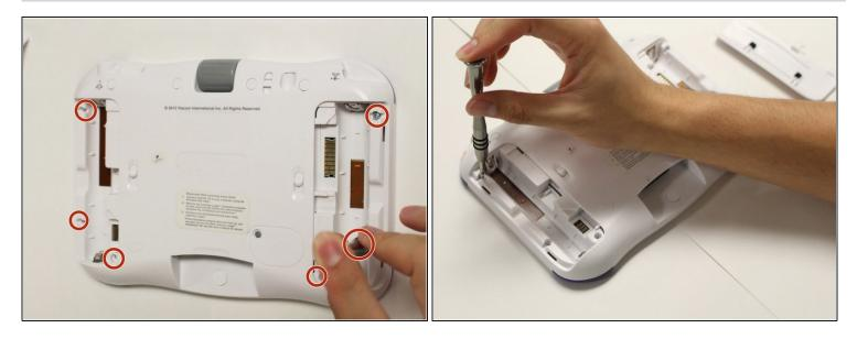
Remove six 7 mm screws from the interior of the battery compartment using a Phillips #1 screwdriver.
