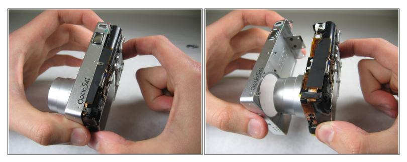
• To remove the front cover, gently hold the inside structure of the camera and slowly pull the front cover off.
