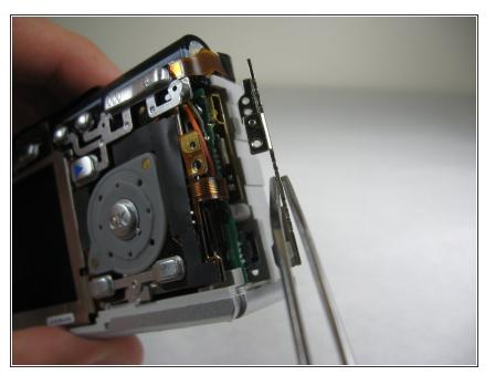
• Pull the cover plate off for the two power cord jacks.
