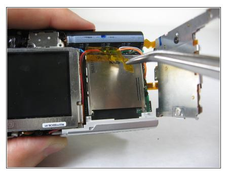
• Remove the orange tape on top of the SD cardholder.
