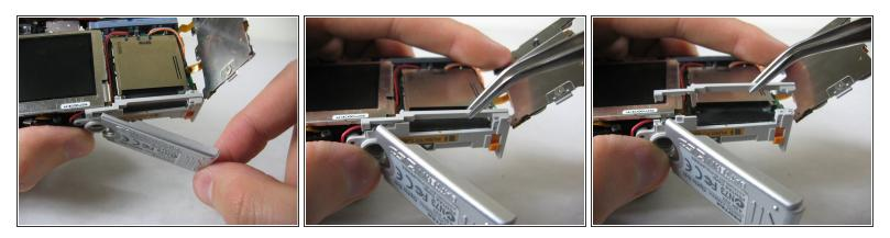
• Open the battery cover and lift plastic piece off.
