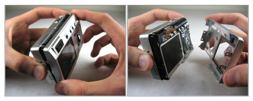
• Carefully pull the back of casing away from the front.
