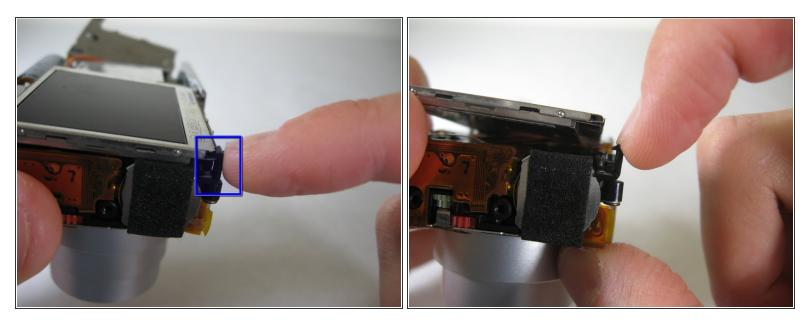
• Push down bottom left LCD bracket to release the LCD from grip.
