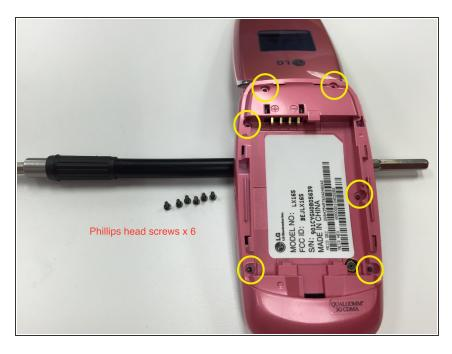
Use the PH000 Phillips-head screwdriver to remove the 6 small screws that were under the battery on the back of the phone. These screws are circled in yellow on the photo.
