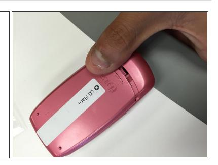
Remove the back cover by pressing down on the raised lines located on the top middle of the back cover and sliding the cover towards the top of the phone.
