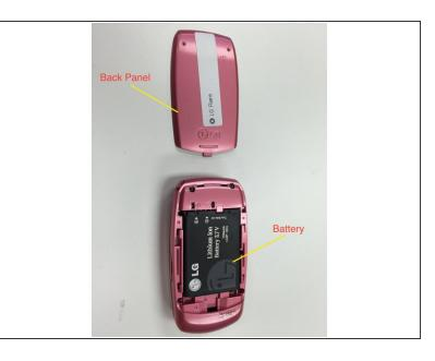
Remove battery by using the smallest of the blue wedges in the iFixit tool kit to lift or pry the battery out of its designated compartment. Place the blue wedge under the battery on the left side (if the LG logo and "Lithium Ion" label are facing toward you) and pry upward to remove.
