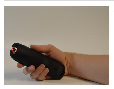
Remove the single 6 mm Phillips #0 screw located beneath the sticker near the USB charging port.
