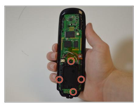
Remove the four 6mm Phillips #0 screws from the battery case.
