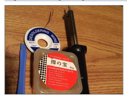
• Gather your solder gun and soldering paste. The soldering paste I use is very cheap and last very long and I apply it with a plastic pry tool, there are other better methods to apply such as the type that comes in a syringe style tube. You will also need desoldering wire or (wick) which conducts heat well and therefore absorbs the old solder.
