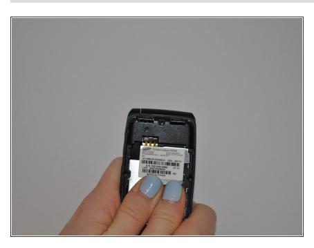
Remove the battery by pressing the battery lock down and slide the battery cover away.
