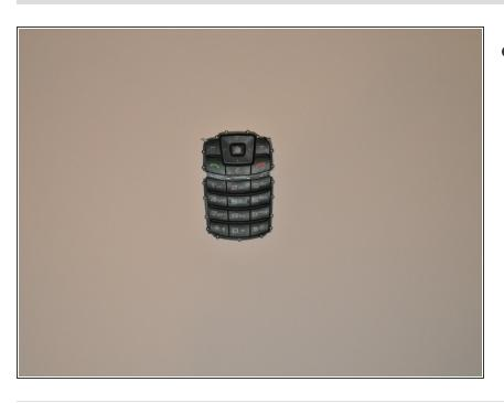
Replace the faulty keypad, and reassemble the phone.
