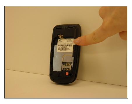
Lift the bottom of the battery and then move it up and away.
