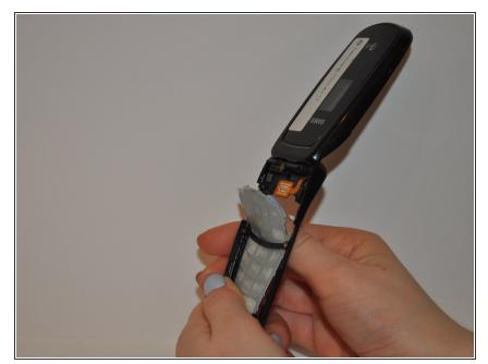
After the connector has been removed you will gently pull off the mother board, which will reveal the rubber keypad.
