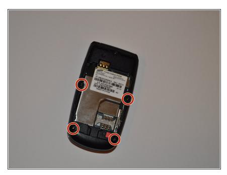
Locate the 4 screws holes on the phone and remove them with the #000 Philips Head screwdriver. (See red circles)
