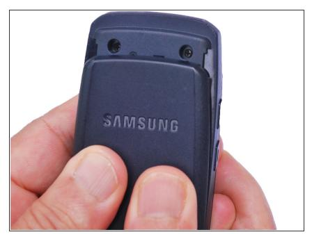
Use your thumbs to pull down on the back cover to remove it and expose the battery.
