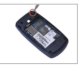
Locate the 4 screw holes and remove the 0.4 mm Phillips head screws using a #000 Phillips head screwdriver. (See red circles)
