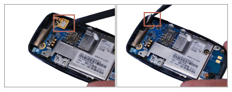
(i) Smaller press-fit connectors may require a simple flick with a plastic opening tool or spudger.
