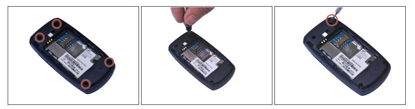
Locate the 4 screw holes and remove the 0.4 mm Phillips head screws using a #000 Phillips head screwdriver. (See red circles)
