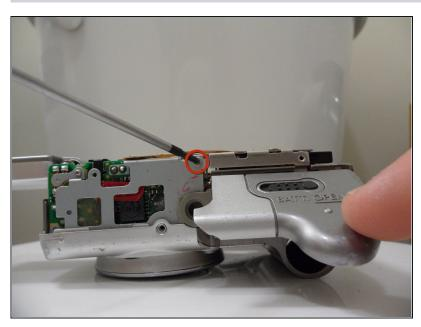
• Remove the marked 2.9mm screw shown.
