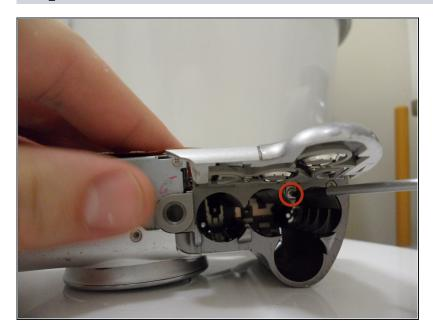
Lift open the battery cover and unscrew the 3.8mm screw as shown.
