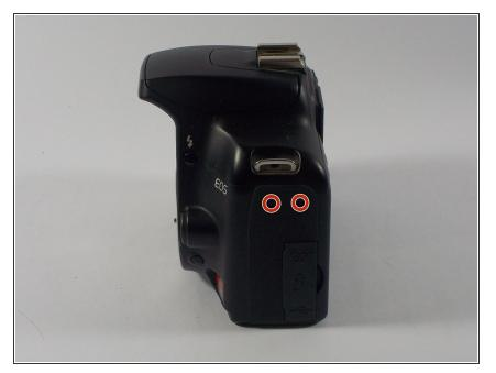
Remove the two 3mm (1/8") black screws from the side cover using a #00 Phillips screwdriver.
