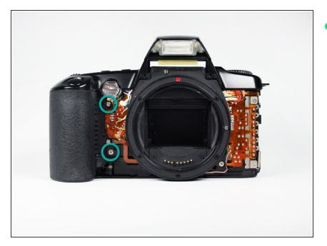
Remove the two 5mm (.20in) long silver screws securing the grip to the camera using a #00 Phillips screwdriver.
