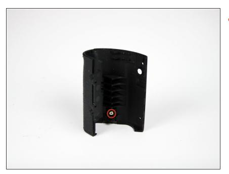
Remove the 4.8mm (.19in) long silver screw from the inside of the grip.
