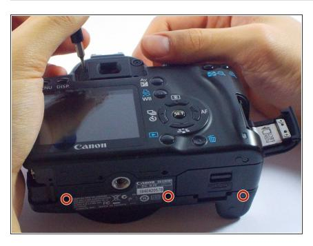
Remove three medium length screws from the bottom of the camera
