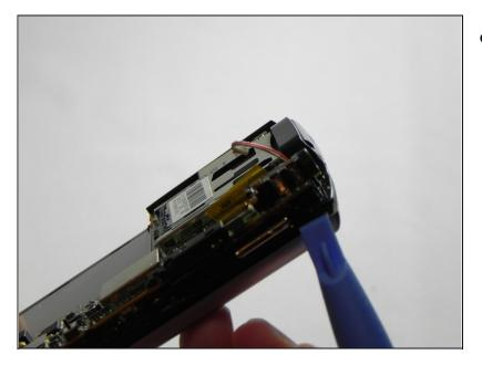
• Next, use a plastic removal tool and separate the silver front case from the black frame.
