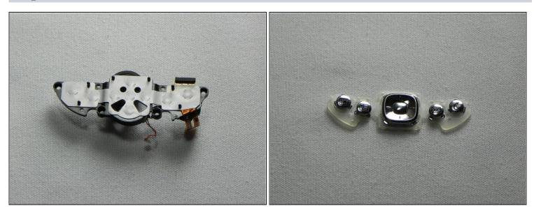
• Once removed you can easily separate the keys from the body.
