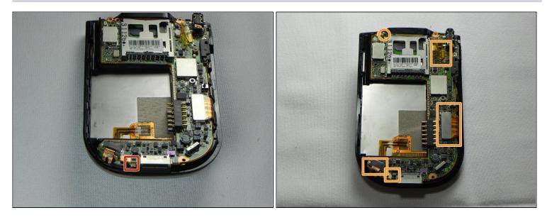
• Next, remove the wire from the bottom of the mother board.
