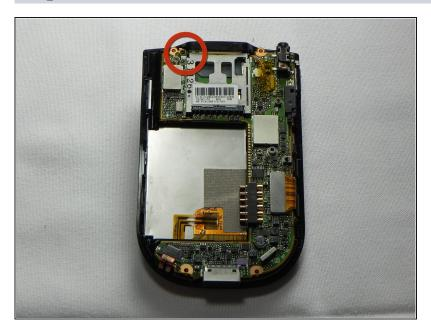
Now that the back cover is removed, use the #00 Philips x .17 screwdriver to remove the small screw to the left of the SD card slot.
