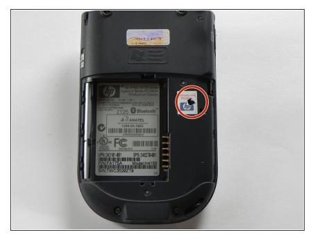
Remove the single black screw that is located beneath the HP sticker with the T5 Torx Screwdriver.
