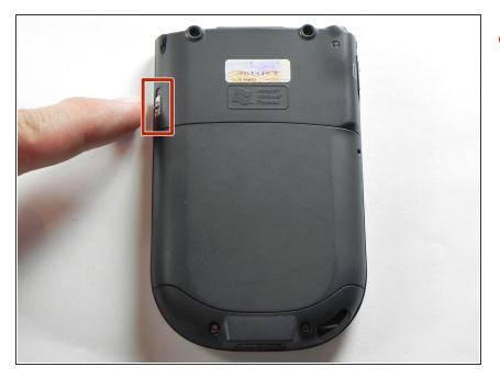
While sliding the silver release tab up, simultaneously lift the cover up from the left side.
