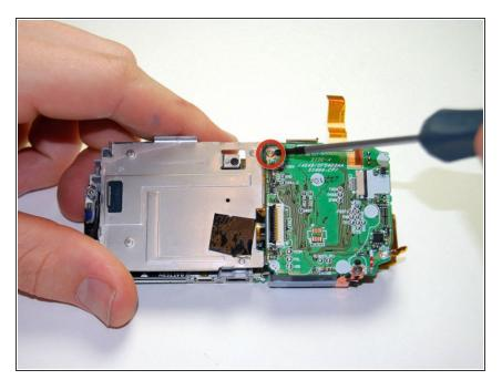
Remove the 2.5 mm silver screw from the upper left corner of the motherboard.
