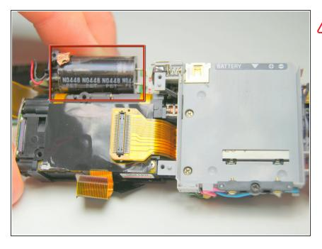
Do not touch the black cylinder on the top edge. This is the capacitor for the flash and it may shock you.
