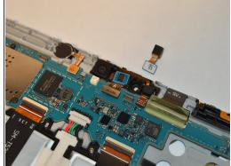
• Use plastic tweezers to carefully detach the front-facing camera from the motherboard.
