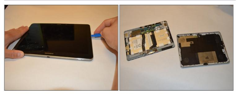
A Be gentle, the front panel is connected to sensitive wiring that may snap if too much pressure is applied.
