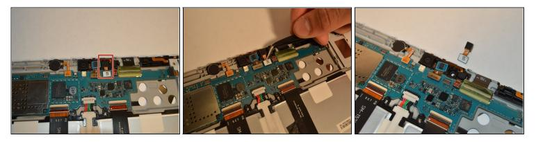
• Use plastic <u>tweezers</u> to carefully detach the front-facing camera from the motherboard.
