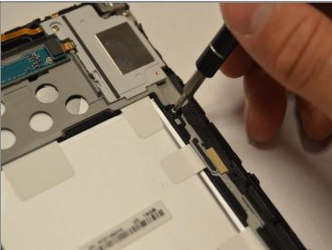
• Remove the six 4 mm Phillips #00 screws that hold the battery in place.
