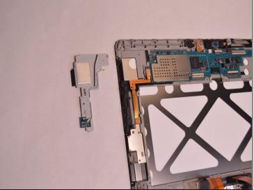
• Remove the Phillips #00 screws from the plastic part holding down the motherboard.
