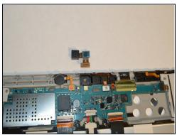
• Use plastic <u>tweezers</u> and carefully detach the rear-facing camera from the motherboard.
