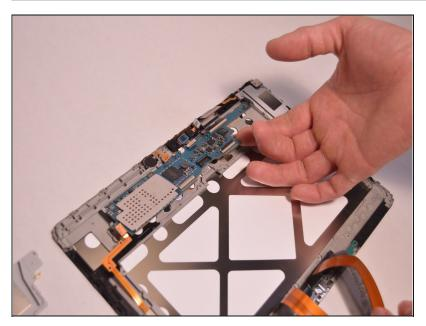
• Gently lift the motherboard from the front panel enclosure.
