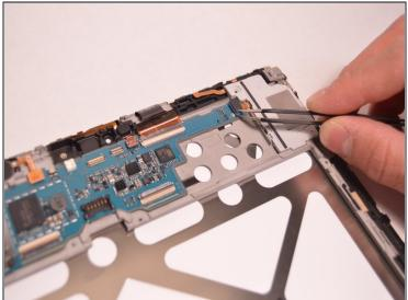
• Remove the five ribbon cables holding the motherboard together with a plastic tweezer.
