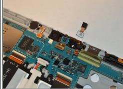
• Use plastic <u>tweezers</u> to carefully detach the front-facing camera from the motherboard.
