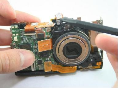
• Use spudger to carefully lift the LED light off the upper-left corner of the lens.
