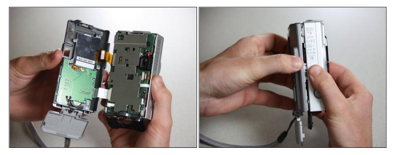
• Carefully slide both halves of the camera together, making sure all tabs are aligned. Press the sides firmly together until you hear a click.
