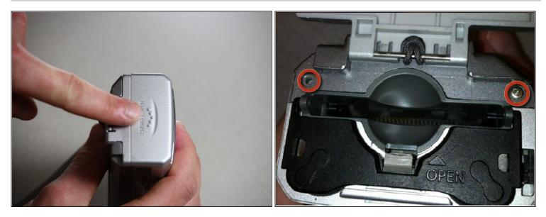
• Open the battery compartment on the right side of the camera by pushing slightly in the direction of the arrow.
