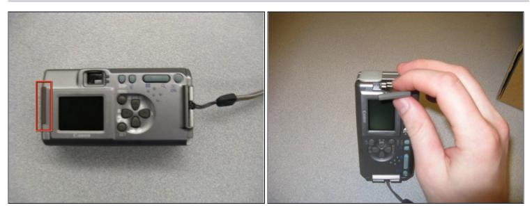
• Remove the screen battery located to the left of the screen.
