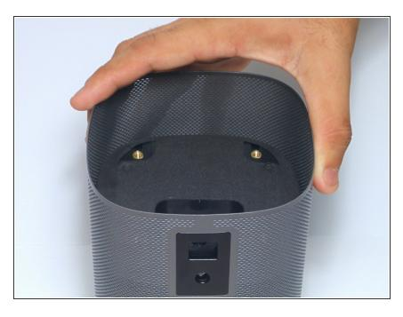
Remove the exterior screen by lifting it away from the bulk of the device.
