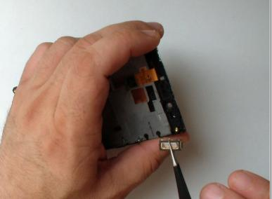
• Use a tool with a sharp point and carefully unstuck the earpiece.
