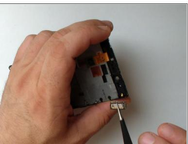
Use a tool with a sharp point and carefully unstuck the earpiece.
