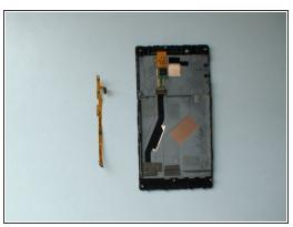
Mhen you start with the removing the ribbon cable be careful with the buttons and with the small black cups on it.
