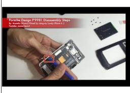
remove the keyboard Connector carefully
