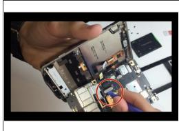
remove the security clasp so u can pull out the screen's ribbon cable carefully
