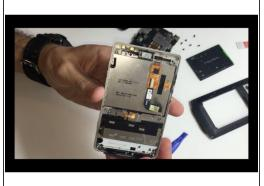
carefully pull out the screen's ribbon cable
