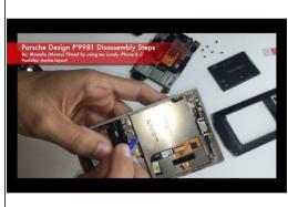
carefully remove the connector of screen keys ribbon cable
