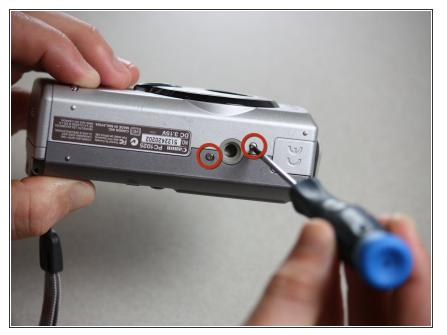
Use a Phillips #00 screwdriver to remove the two screws at the bottom of the camera.
