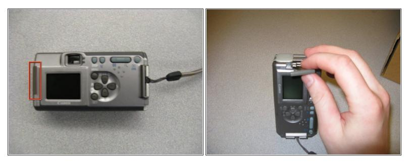
• Remove the screen battery located to the left of the screen.
