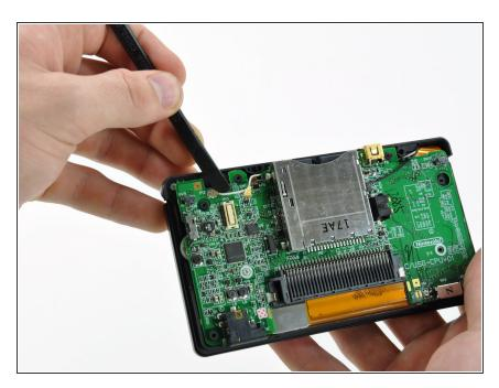
Use the flat edge of a spudger to pry the microphone connector straight up from its socket on the motherboard.
