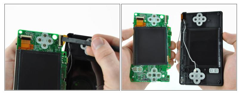
• Use your fingernail or the flat edge of a spudger to carefully flip up the upper LCD ribbon cable retaining flap.
