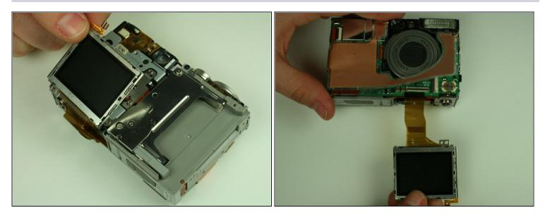
• Remove the LCD screen and set it aside.
