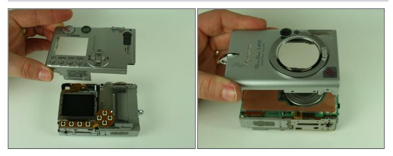
A When removing the casing, do not drop the small black plastic piece. This piece sits in a small gap above the lens, to the left of the flash, and underneath the camera case.
