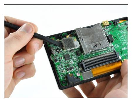
Use the flat edge of a spudger to pry the Wi-Fi board connector straight up from its socket on the motherboard.
