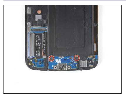
• Remove the two 2.5mm Phillips #00 screws.
