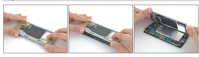
• Press down on the back of the battery and lift up on the edges of the midframe to separate it from the rest of the phone.
