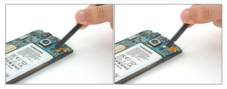
• Using the flat end of the spudger, disconnect the battery ribbon cable from the motherboard.
