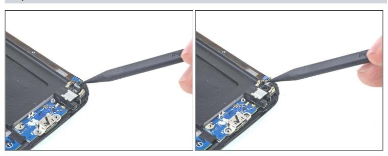
• Using the pointed end of spudger, pry up the small section of daughterboard secured with a light adhesive.
