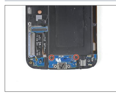
Remove the two 2.5mm Phillips #00 screws.
