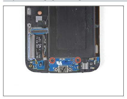
Remove the two 2.5mm Phillips #00 screws.
