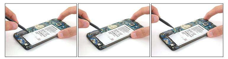
• Use the pointed end of a spudger to disconnect the two antenna interconnect cables from the motherboard.
