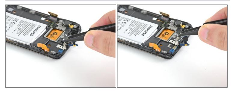
• Remove the EMI shield that covers the proximity and gesture sensors.
