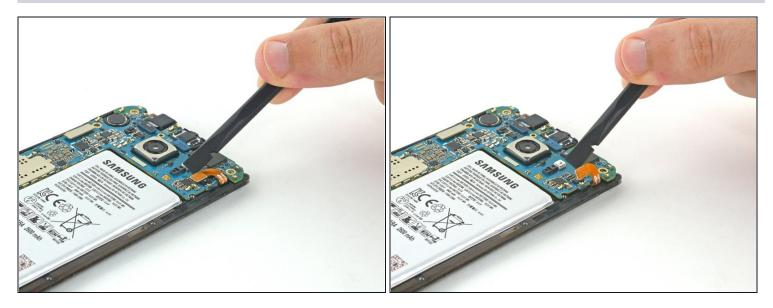
• Using the flat end of the spudger, disconnect the battery ribbon cable from the motherboard.
