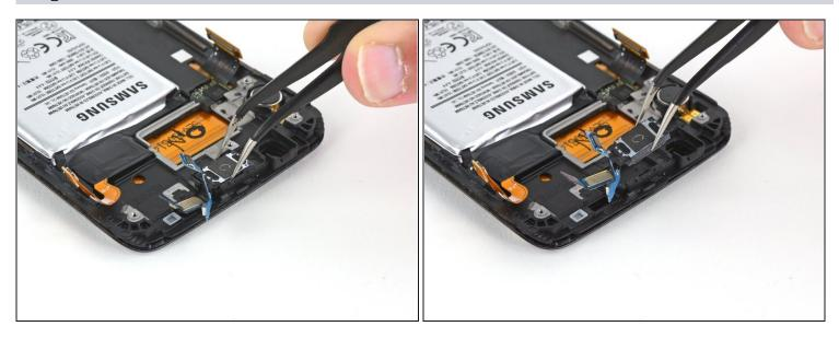
• Pull the earpiece speaker assembly out of the phone, taking care not to strain any cables.
