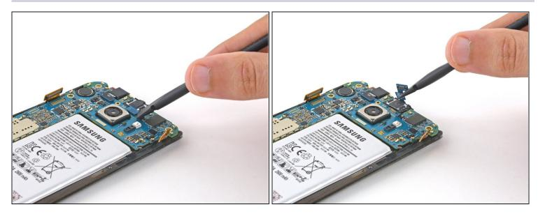
• Disconnect the earpiece ribbon cable from the motherboard.
