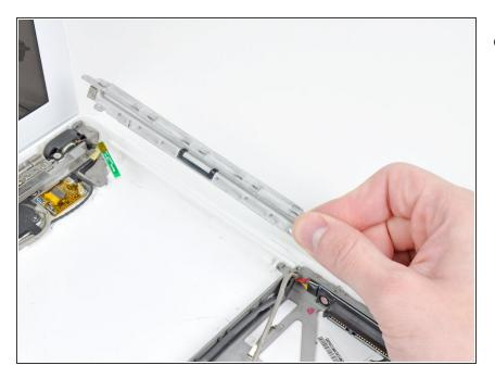
• Remove the optical drive bezel from the lower case.
