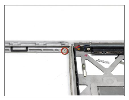
Remove the single 3.1 mm Phillips screw below the inside of the optical drive opening.
