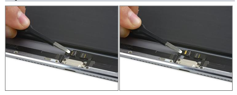
• Slide the left speaker cable out of its ZIF connector.
