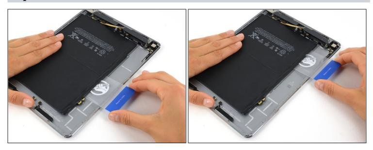
• Slide the plastic card up along the edge of the battery until the card is even with the top edge of the battery.
