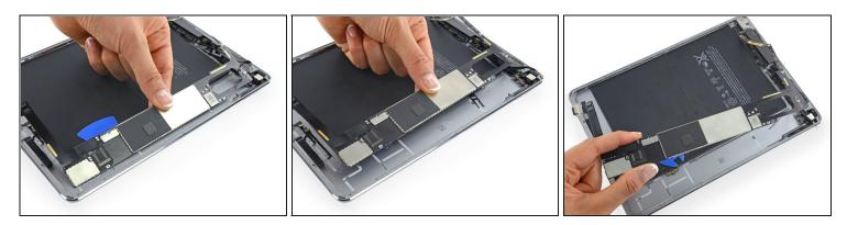
• Remove the logic board.
