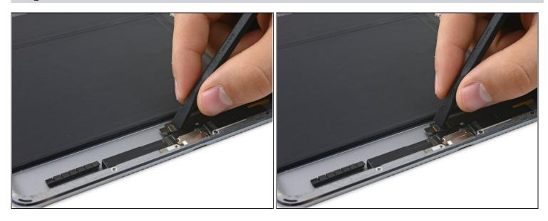
• Use a spudger to flip up the retaining flap on the left speaker's ZIF connector.
