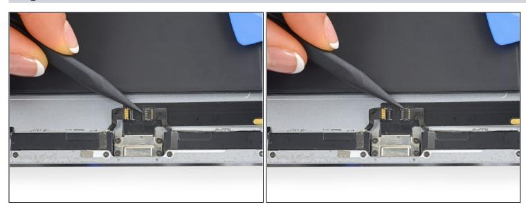
• Use a spudger to flip up the retaining flap on the right speaker's ZIF connector.
