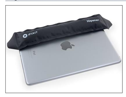
Place a heated iOpener on the lefthand side of the back of the iPad for 2-3 minutes.
