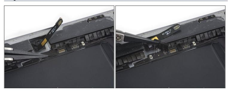
• Peel up the tape covering the top left edge of the logic board.
