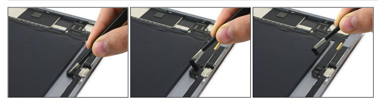
Remove the tape covering the two speaker ZIF connectors.
