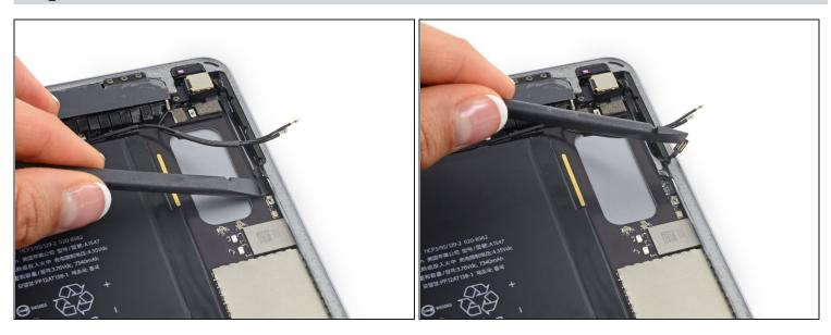
• Detach the volume button cable connector by prying it straight up from its socket.
