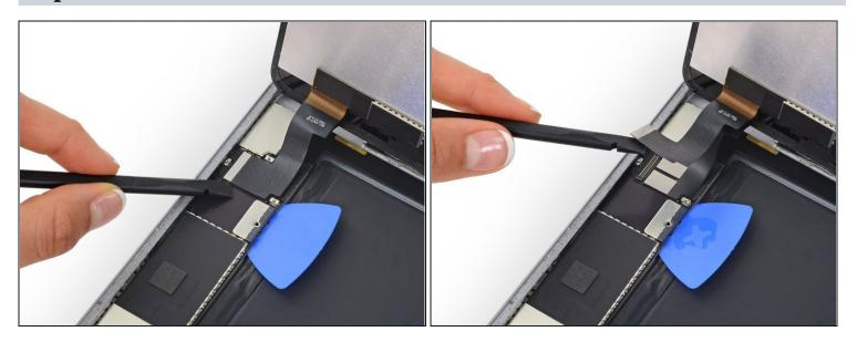
• Disconnect the display data connector from its socket on the logic board.
