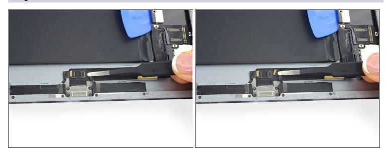
• Slide the right speaker cable out of its ZIF connector.
