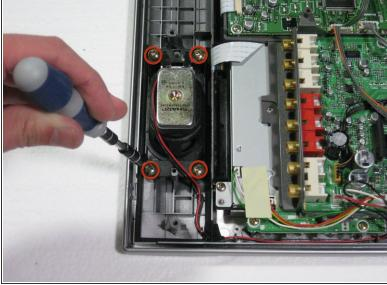
• Remove the eight 9mm screws from both speakers.
