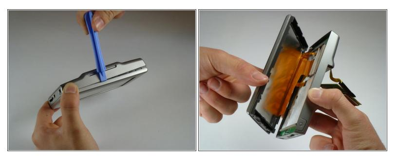
Gently pull apart the front and back of the device. The front and back are still connected by ribbon cables.
