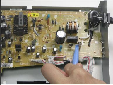
• Using the plastic opening tool, gently pop the fuse out of its restraining brackets.
