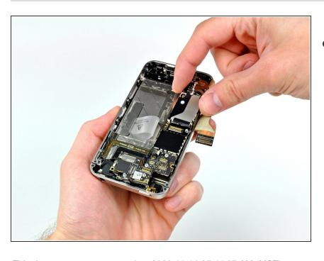
The logic board can finally be lifted out of the iPhone.
