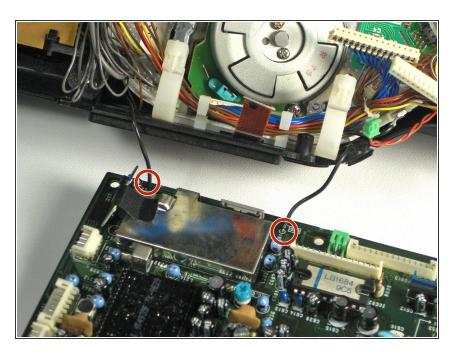
Desolder the two black wires holding the motherboard to the camcorder using a soldering iron.
