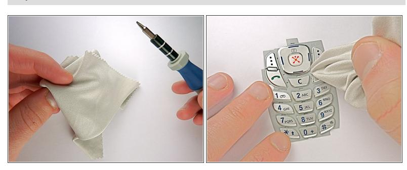
By using a small standard screwdriver and a fine, thin, soft cloth you can clean in between the keypad to remove dirt and debris.
