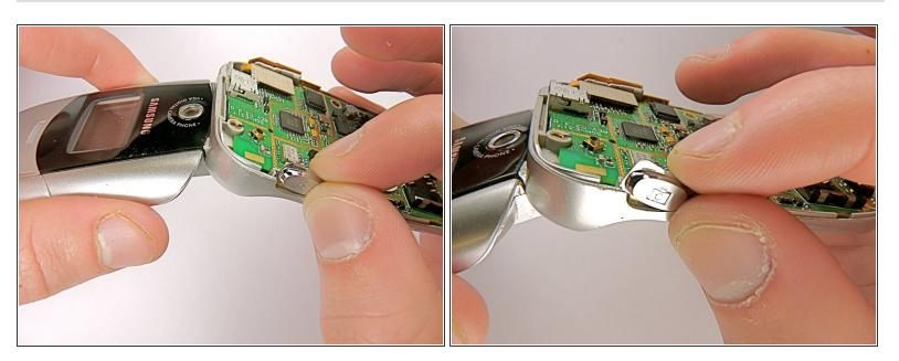
Remove the camera and volume buttons and place them in a safe spot until reassembly.
