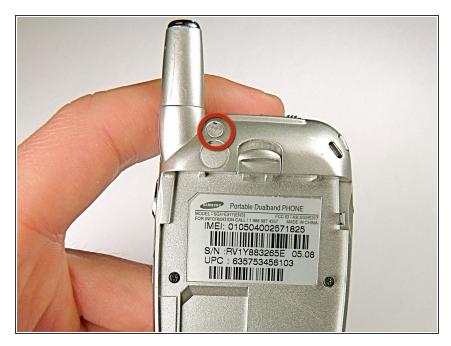
Remove the rubber screw cover using your fingernail.
