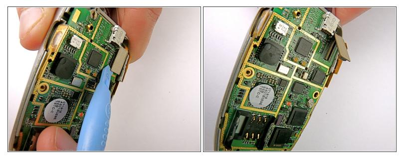
Using a plastic opening tool, unplug the ribbon cable connecting the front LCDs to the motherboard.
