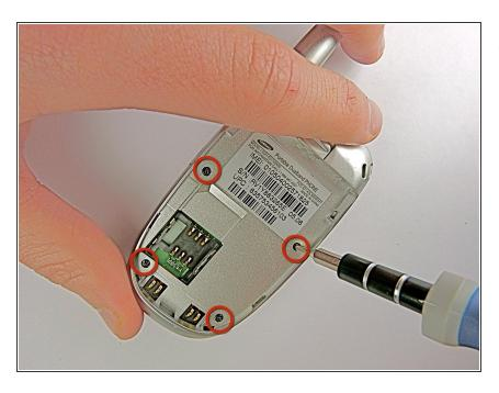
Unscrew the four 4.5mm screws located on the back plate.
