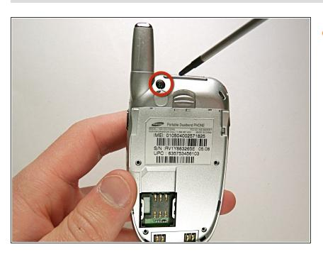
Unscrew the 4.5mm screw located underneath the rubber cover.
